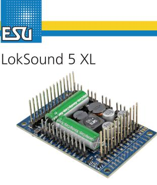
The LokSound 5 XL decoder is an extremely powerful decoder! It must be as it is intended for use in your garden railway or 1/G gauge locomotives. Its integrated, power-adapted PowerPack ensures safe operation even on dirty tracks.
