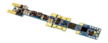
The LokSound 5 micro DCC Direct Kato USA has been specially developed for installation in N gauge locomotives of the Kato USA brand: Most diesel locomotives of this manufacturer are installed in the American model of these decoders instead of the analog board installed as standard. Finally, these models can also be easily retrofitted with a LokSound decoder.
