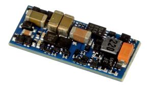
With the LokSound 5 Nano DCC, ESU has succeeded in developing an even smaller LokSound decoder: With only 19.6 mm x 8.5 mm x 3.2 mm, it is the smallest LokSound decoder we have ever built. Thus, it should really be used in all vehicles of nominal sizes N and TT.
