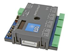
SwitchPilot 3 decoders are optimized for stationary use on your system and can switch conventional double coil switch drives, light signals, magnetic uncouplers, light bulbs or other stationary consumption.In order to facilitate the rather cumbersome configuration of magnetic article decoders, the SwitchPilot 3 has an innovative operating concept consisting of a 4-line, illuminated OLED display and three input buttons.
