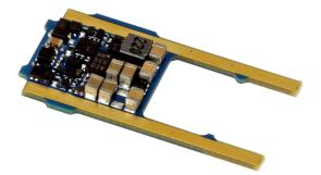
The LokSound 5 micro DCC Direct Kato Japan has been specially developed for installation in Kato-branded N gauge locomotives: in many European and Japanese locomotives of this manufacturer, the ser decoder can be installed directly below the engine instead of the analog board installed as standard. Finally, these models can also be easily retrofitted with a LokSound decoder.
