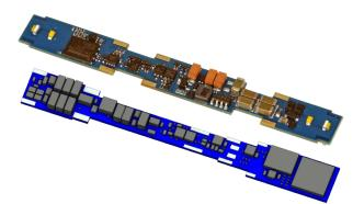
The LokSound 5 micro DCC Direct has been specially developed for installation in N gauge locomotives of the Atlas and Intermountain brands: it can be inserted directly instead of the analog board installed there as standard. However, the decoder can also be used for similar models from other manufacturers at your own discretion.
