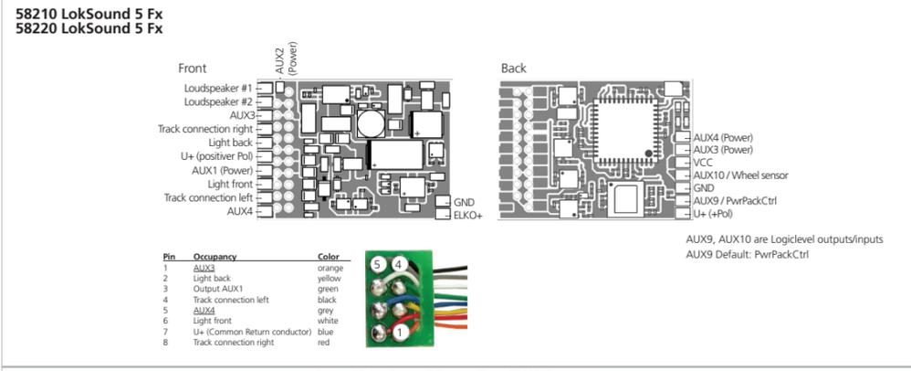
Figure 10: LokSound 5 Fx with 8-pin NEM652 interface
