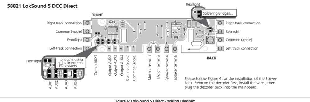
Figure 6: LokSound 5 Direct - Wiring Diagram
