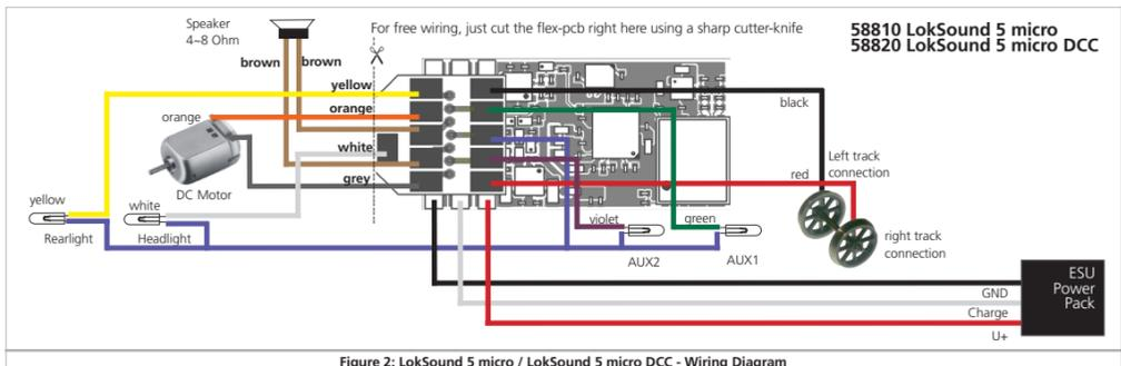
Figure 2: LokSound 5 micro / LokSound 5 micro DCC - Wiring Diagram
