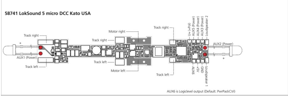
Figure 4: LokSound 5 micro DCC Kato USA
