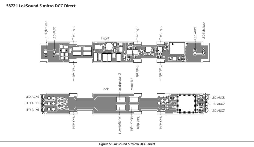
Figure 5: LokSound 5 micro DCC Direct
