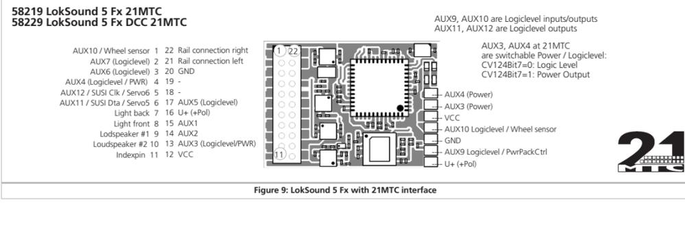
Figure 9: LokSound 5 Fx with 21MTC interface
