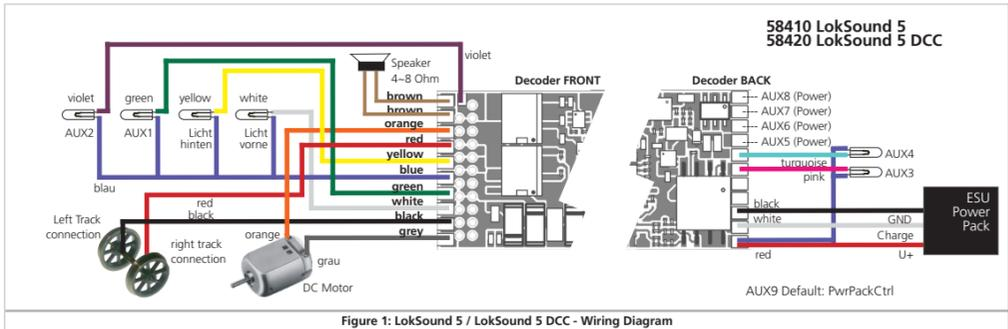
Figure 1: LokSound 5 / LokSound 5 DCC - Wiring Diagram
