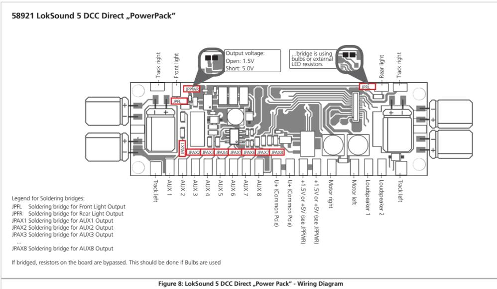
Figure 8: LokSound 5 DCC Direct „Power Pack“ - Wiring Diagram
