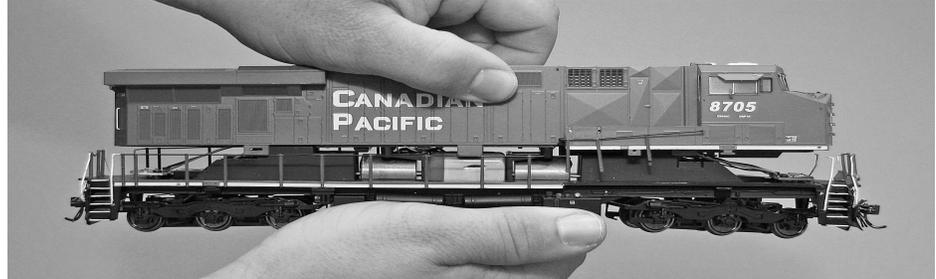
To remove the shell, firmly grip the fuel tank area and the center area of the body. Gently rock the shell side to side to release the holding tabs and lift straight up. Watch that the handrails do not get caught on the body deck or cab while being lifted off.
