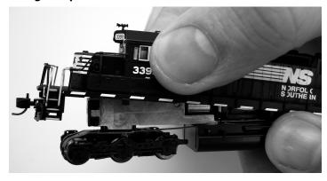
Once the shell is off you will see the decoder on top of the die-cast chassis. If you need to remove the decoder for any reason, sliding it forward gently will release it from the die-cast contacts. The decoder can only be installed one way so if it doesn't slide back in easily, don't force it. Check that it is oriented correctly and carefully try again.
