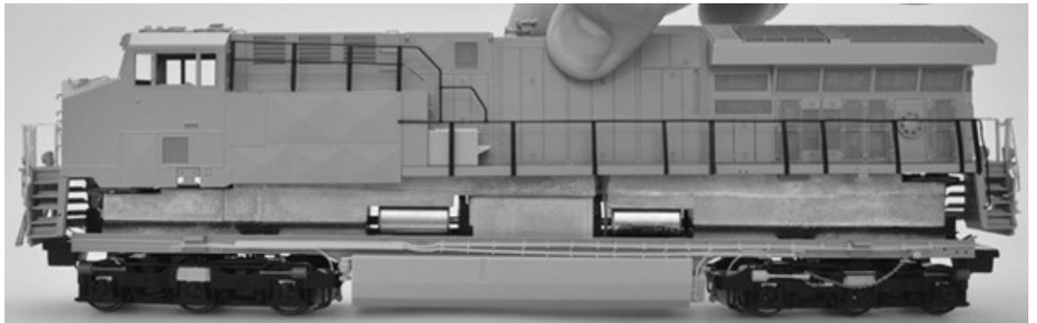
4. The shell should slide off of the chassis to reveal the mechanism and electronics. There are no wires attaching the shell to the drive.
