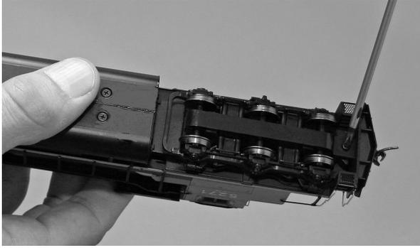
1. Place the locomotive on a soft surface or foam cradle. Remove the front and rear couplers from the locomotive. Utilize a Philips head screw driver to unscrew the coupler from the frame. Gently slide the coupler box from the shell and frame. The coupler box may need to be disassembled in place and removed as separate pieces. Keep the pieces together for re-assembly.
