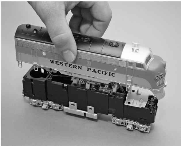
4. The chassis should drop out of the shell to reveal the mechanism and electronics.
